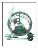
**1-SR130B** Super Reach 130 Brush System (Hydmaster 40) ... \$14,995.00 Electric/hydraulic (more torque) brushing system
