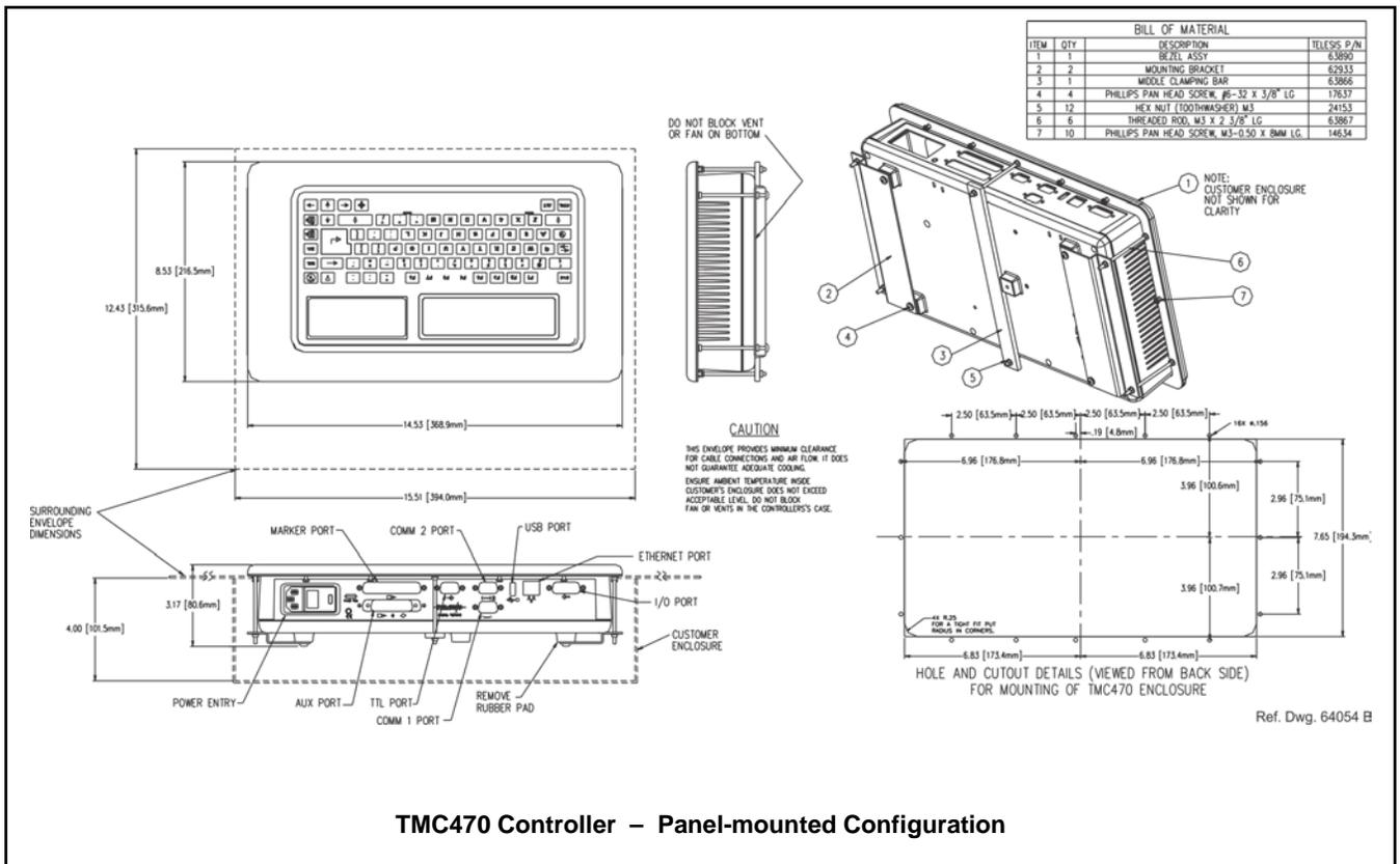
**TMC470 Controller – Panel-mounted Configuration**
