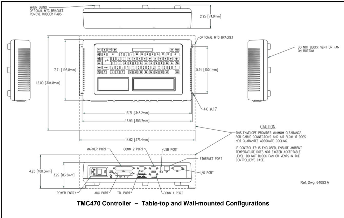
**TMC470 Controller – Table-top and Wall-mounted Configurations**
