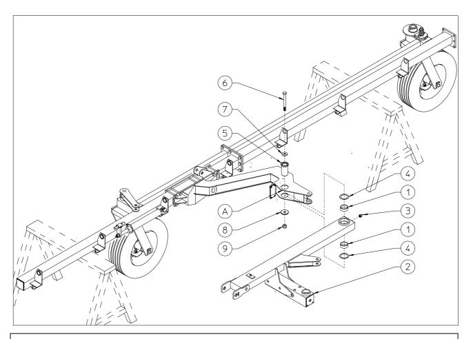
Attach the nylon bushings 1 to the proper seats. Attach the grease nipple 3 to the proper seat.
