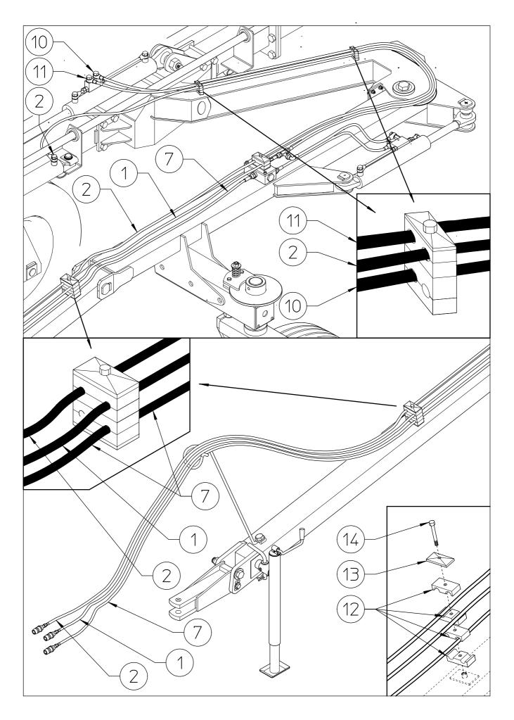
Fasten the hoses 1-2-7 using hose collars 12, plate 13 and screw 14. Fasten the hoses 2-10-11 using hose collars 12, plate 13 and screw 14.
