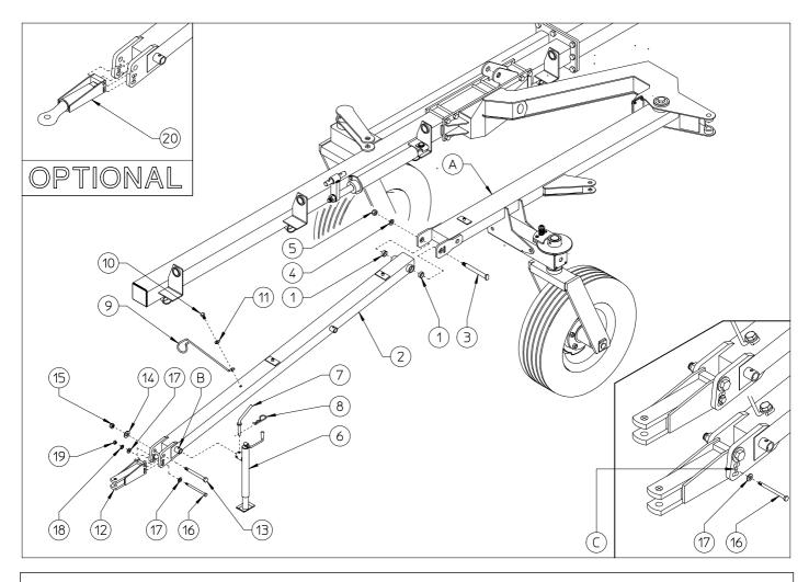
Attach the bushings 1 to the proper seats. Now attach drawbar 2 to support A using pin 3, washer 4 and nuts 5. Attach the stand 6 to seat B on drawbar 2 using the pin 7 and clip 8. Assemble the hose support 9 with the screw 10 and nut 11.
