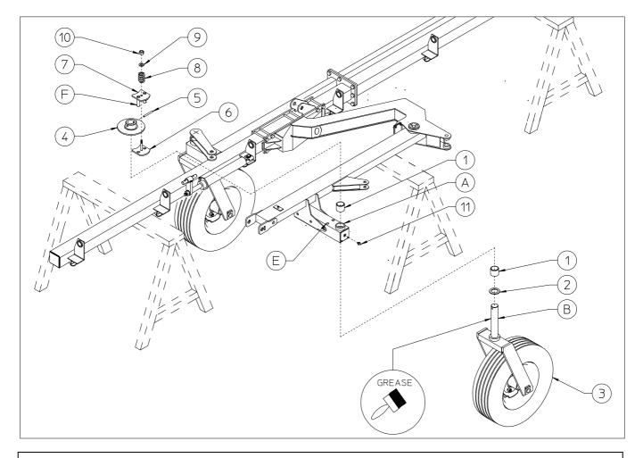
Before attaching the wheel unit 3, brush pin B and spring pin 5 with grease.
