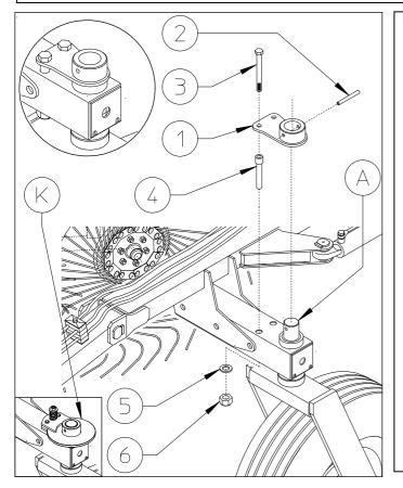
Moreover when working on sloping ground, the machine tends to lose the right set of work. In these cases it could be helpfull to assemble a kit **(OPTIONAL)** that goes to lock the oscillation of wheel 6.
