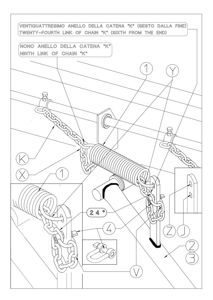
Hook X on spring 1 is more closed than hook Y. Hook Y (the more open one) should be inserted into hole Z in the lever of arms 2-3 (RH-LH).
