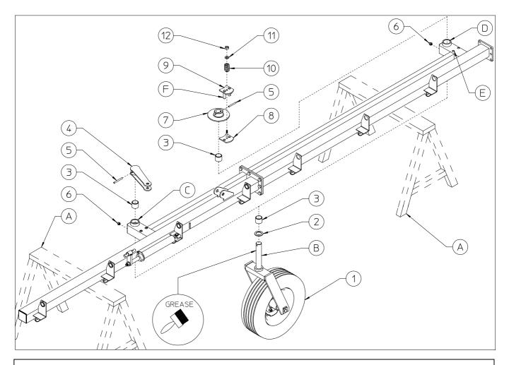
Before attaching the wheel units 1, brush pin B and spring pins 5 with grease.
