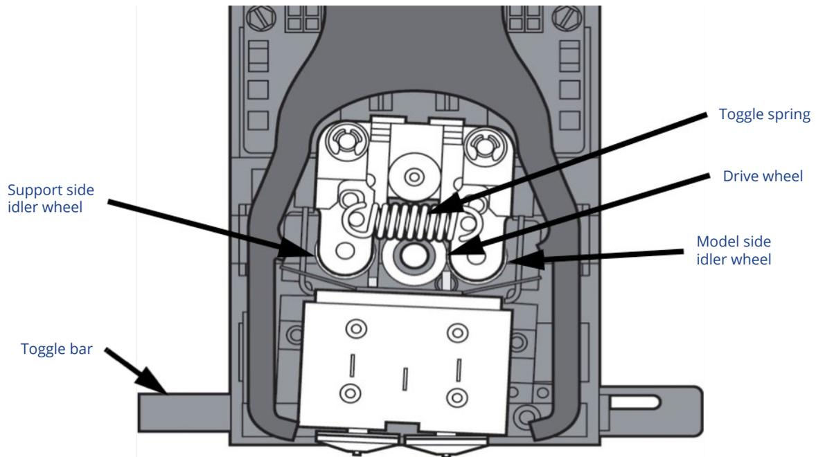
**Figure 6:** Toggle bar in neutral position
