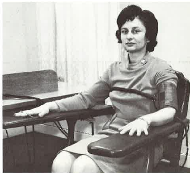
Subject being tested sits in this chair while answering questions. Tube around chest measures rate of respiration, cuff on arm measures blood pressure, and rings attached to fingers of right hand measure galvanic skin response.
