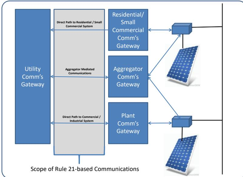
**Figure 2: Scope of CA Rule 21 DER Communications**
