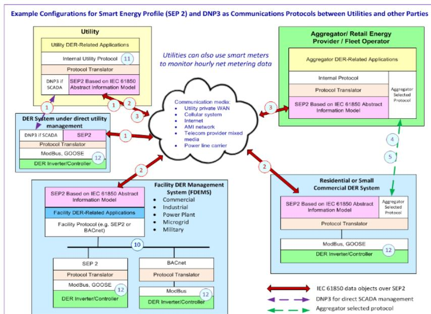
Figure 3: Conceptual Implementation of IEEE 2030.5 (SEP2) Communications with DER<sup>12</sup>
