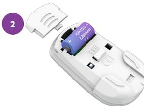
Open the battery cover and insert the battery
