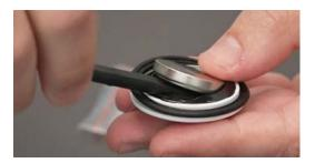
5. Place the new battery in the upturned front section of the device with the + sign facing up.
