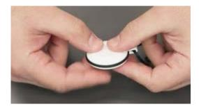
8. Hold the two sections together gently and turn the device the correct way up, making sure that the rubber seal stays in place.
