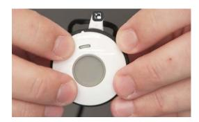
9. Align the point on the front section of the device with the dot on the back section.
