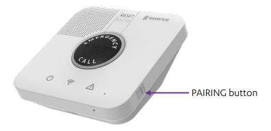
The control panel beeps and the ring around the **EMERGENCY** button lights up in blue with a circular movement effect.
