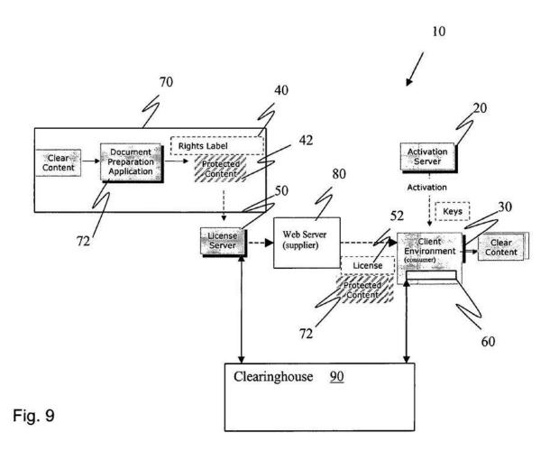
Figure 9 is block diagram of a DRM system 10 that enforces usage rights and meta-rights for specific content and services. *Id.* at 2:15–18. A user activation component (server 20) issues public and private key pairs, or other identification mechanisms, to content users. Software, installed in client 30 associated with the content recipient, enforces usage rights for protected content. Client component 60 contains public and private keys issued by activation server 20. *Id.* at 4:20–35.
