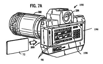
Figure 7A depicts "a hand[-]held device for capturing, storing, and transmitting an image in accordance with the invention." *Id.* at 4:46–48, 11:3–20.
