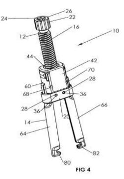
Figure 4 is an isometric view of the rod reducing device with the screw jack mechanism fully retracted and the two elongated grasping members in an open configuration. Ex. 1001, 3:2–32.
