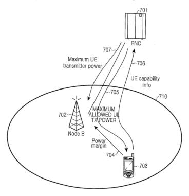
Figure 7 depicts UE 703, RNC 701, and Node B 702. *Id.* at p. 12, ll. 23–29. Node B 702 receives Tx power 704 from UE 703, receives maximum UE transmitter power 707 (of UE 703) from RNC 701, and uses those values to "calculate the Tx power margin of the UE 703" using the equation above. *Id.* at p. 12, l. 23–p. 13, l. 8.
