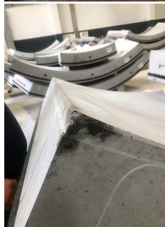
..... Over-applied mineral oil left to accumulate in the bottom of a mould.
