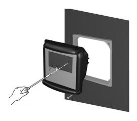
Place the instrument inside the frame and secure it with the M4  $\times$  25 screws. Tighten the screws until the instrument is firmly fixed.
