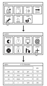
To activate add-ons, select the symbol SYSTEM in the main menu, and in the submenu the symbol ADD-ON.
