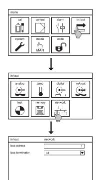
Select the symbol IN/OUT in the main menu and in the submenu, select the symbol NETWORK. Here you can set the following parameters:
