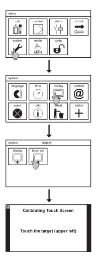
To calibrate the touch screen, select in submenu SYSTEM -> DISPLAY the symbol TOUCH CAL to start the calibration. The touch screen calibration texts are available in English only.
