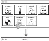
If the datalog add-on is activated, four symbols appear. In the menu LOG PARA you define which parameters you want to log. In LOG SET you define interval and log mode, and view the log status.
