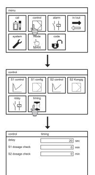
Select CONTROL in the main menu, and in the control menu the symbol TIMING. In this you can define three important times for the controller:
