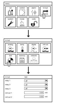
Set the mode to manual. Select the symbol TEST in the submenu  $\ensuremath{\mathsf{IN/OUT}}$ .
