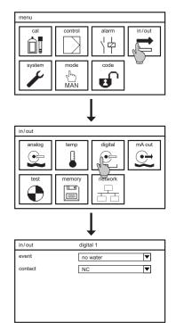
In the entry-level version, the Neon® instrument has one digital input. All settings concerning the digital input(s) are found in the submenu IN/OUT -> DIGITAL. If you have two digital inputs, separate symbols will appear for them.
