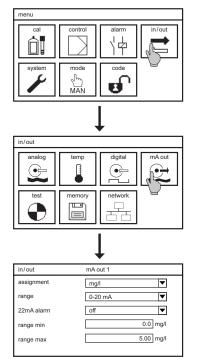
Select the symbol IN/OUT in the main menu and then select the symbol mA OUT. Here you can set the following parameters:
