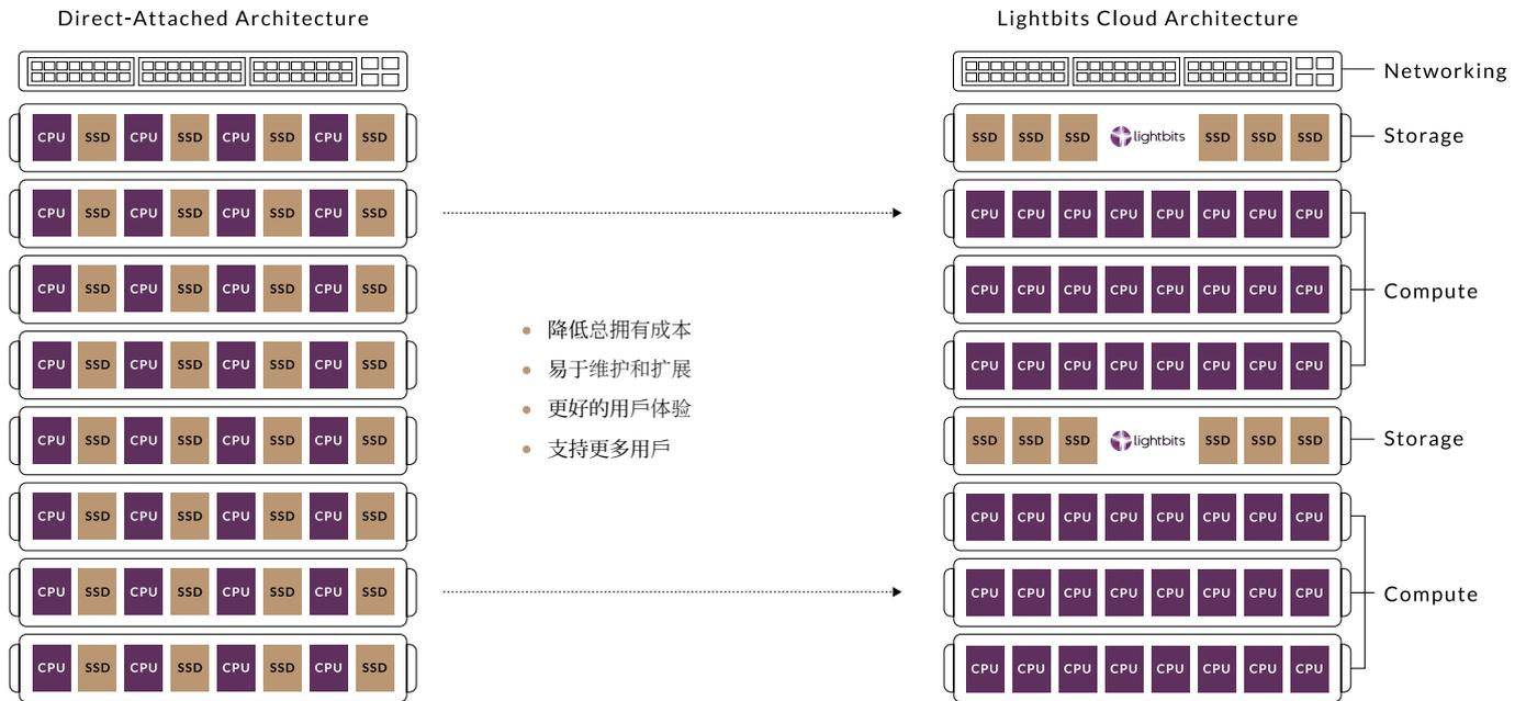
Figure 2: Moving from Direct Attached Storage (DAS) to disaggregated storage and compute
