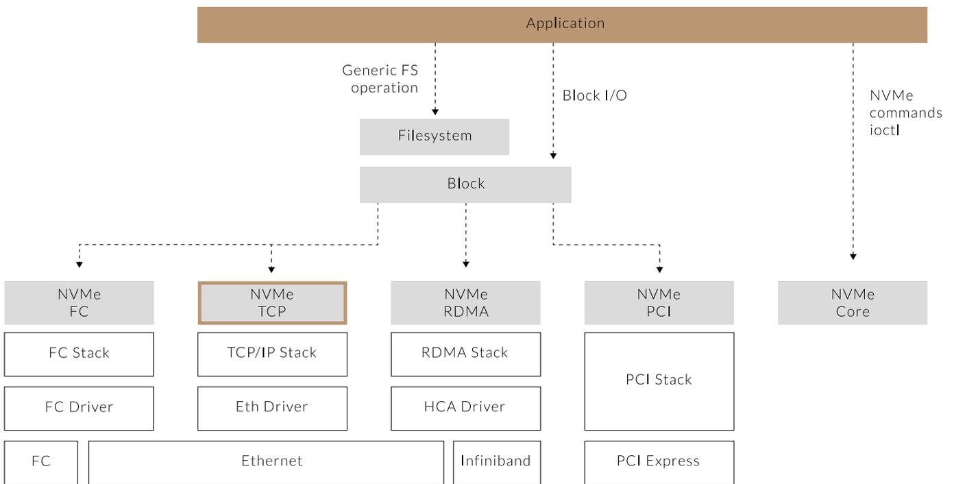
Figure 1: NVMe/TCP seamlessly integrated with existing NVMe protocols in the Linux kernel
