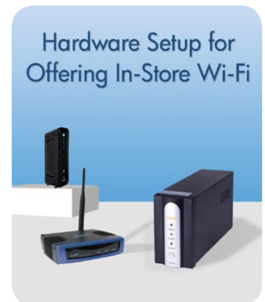
Cable modem (or other type of network connection), wireless access point (AP), and uninterruptible power supply (UPS)
