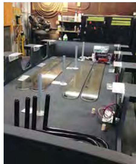
Cutting Edge Composites in Summerville, S.C., fabricated the carriage bodies using resin transfer molding. The bodies are then fastened to steel chassis.
