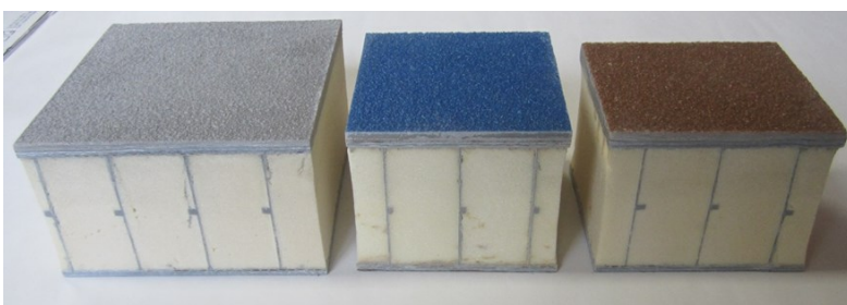
(left) The quartz aggregate is available in a wide range of colors. (below) Patterns are easily created by masking off selected areas and applying a second color once the first color is cured.
