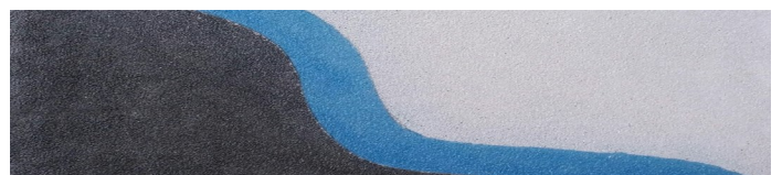
(left) The quartz aggregate is available in a wide range of colors. (below) Patterns are easily created by masking off selected areas and applying a second color once the first color is cured.
