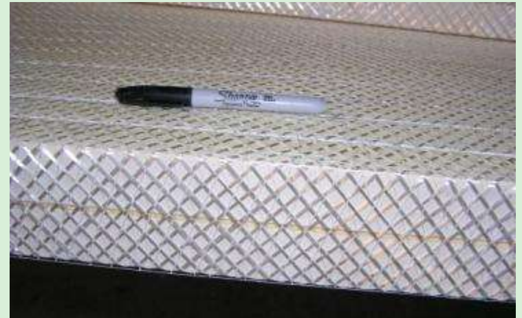
Internal core with fibers for shear
