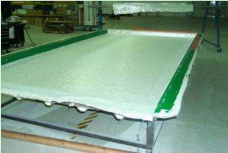
Fiberglass layers in molding tool
