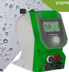
The PRISMA diaphragm and stepper motor metering pump is designed for applications requiring high precision dosing volumes and reliable repeatability. Thanks to the microprocessor controlled stepper motor and excellent pitch resolution of 1: 4800, the entire stroke and suction cycle is controlled with maximum precision.
