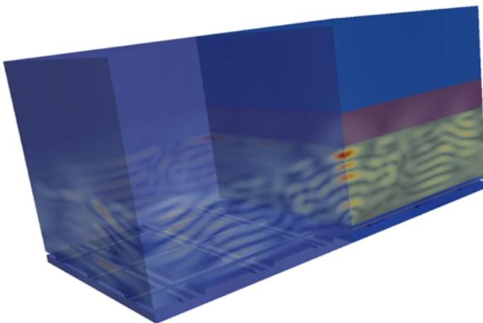
Figure 2: 3D simulation of an ultrasonic sensor fingerprint (Source: OnScale)
