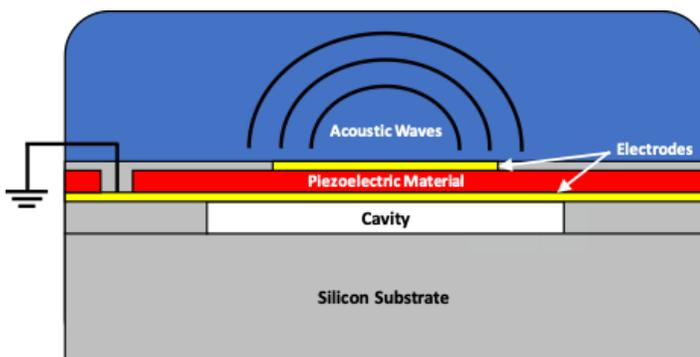
Figure 4: Basic PMUT cell structure (Source: OnScale)
