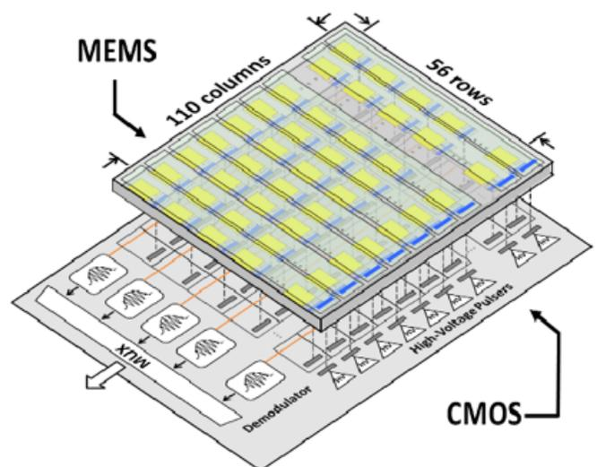
Figure 1: An integrated ultrasonic fingerprint sensor (Source: Horsley et al)<sup>1</sup>
