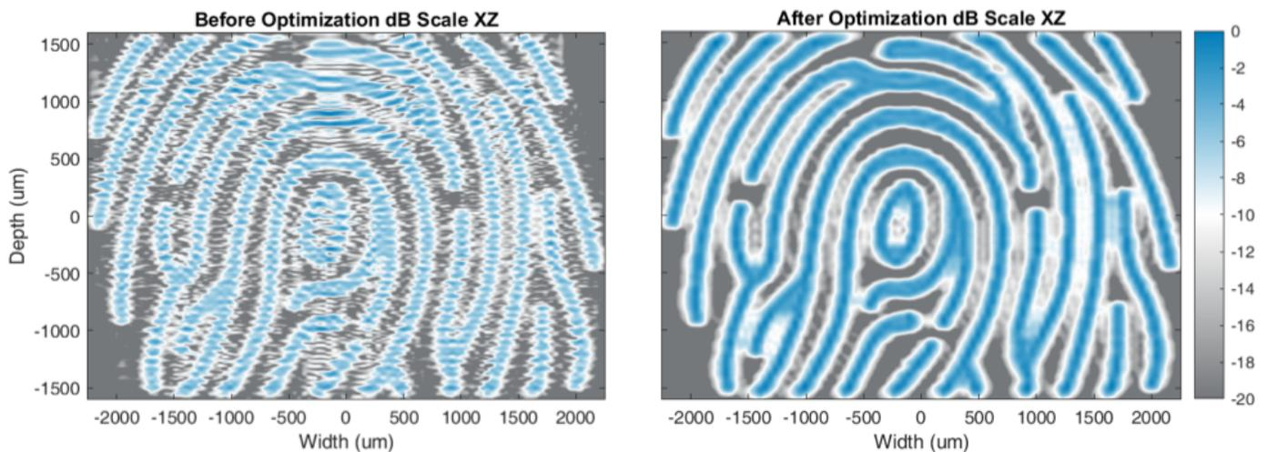
Figure 8: Virtual fingerprint image before (left) and after (right) beamforming optimization
