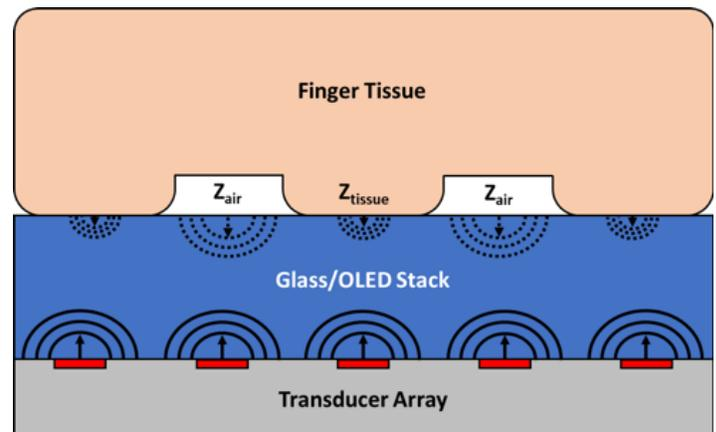
Figure 3: Ultrasonic fingerprint technology (Source: OnScale)
