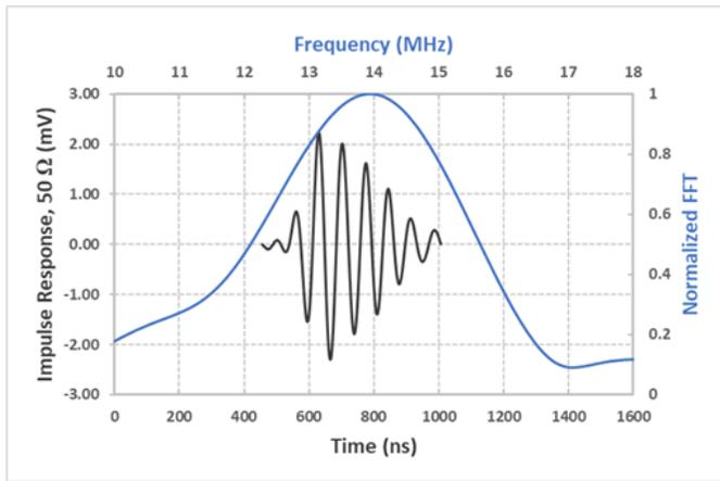
Figure 7: Pulse-echo response of a single PMUT column
