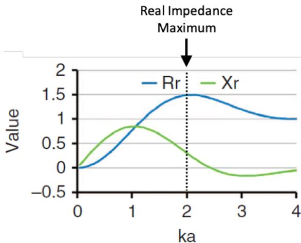
Figure 6: Radiation impedance as a function of wave number and lateral size (Source: Jiang et al)<sup>5</sup>
