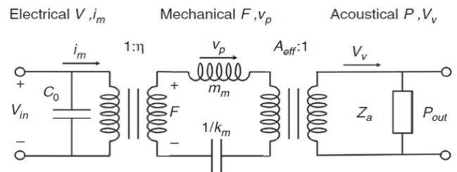
Figure 5: Lumped-element small signal PMUT model (Source: Jiang et al)<sup>5</sup>
