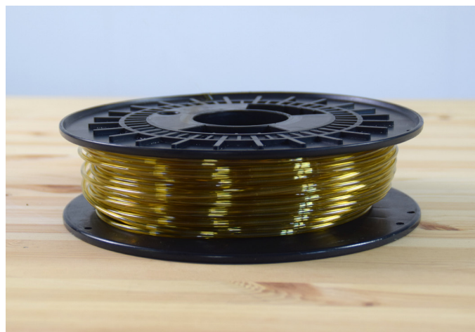
A custom-made roll of PEKK filament, efficiently extruded by the NEXT. Before buying the NEXT, ESA's Spaceship EAC team sourced filament from third-party suppliers. Now, they make their own materials in-house, thus reducing lead-times and retaining control over research and prototyping.
