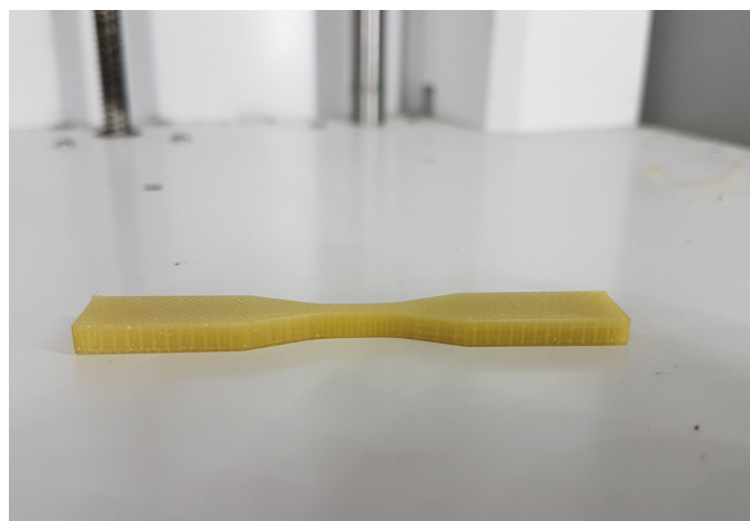
Spaceship EAC regularly uses 3D printing for product and system prototyping. Here, a 3D printed specimen is ready for analysis.
