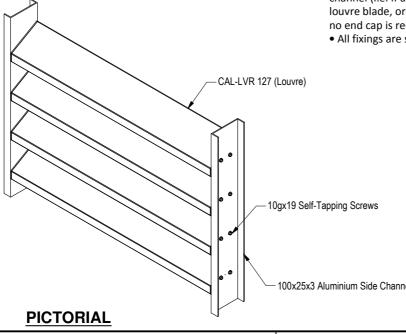
Not sure if this is the correct fixing detail for your project? Contact Aurae to discuss your requirements -we will be able to recommend the 100x25x3 Aluminium Side Channel most suitable fixing methods for your specific scenario.
