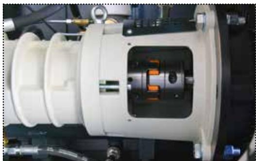
BLADE 8-12 has been designed in a way that makes it possible **to replace the elastic element** without having to dismantle the rotor-stator unit.
