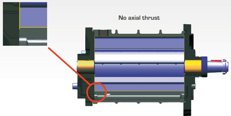
**Fig. 9** - There is no axial thrust in a rotary vane compressor. The rotor is free to move axially and is kept equally spaced from the end covers by means of the lubricant, which is injected under pressure. The injected lubricant prevents the air from escaping along the side planes
