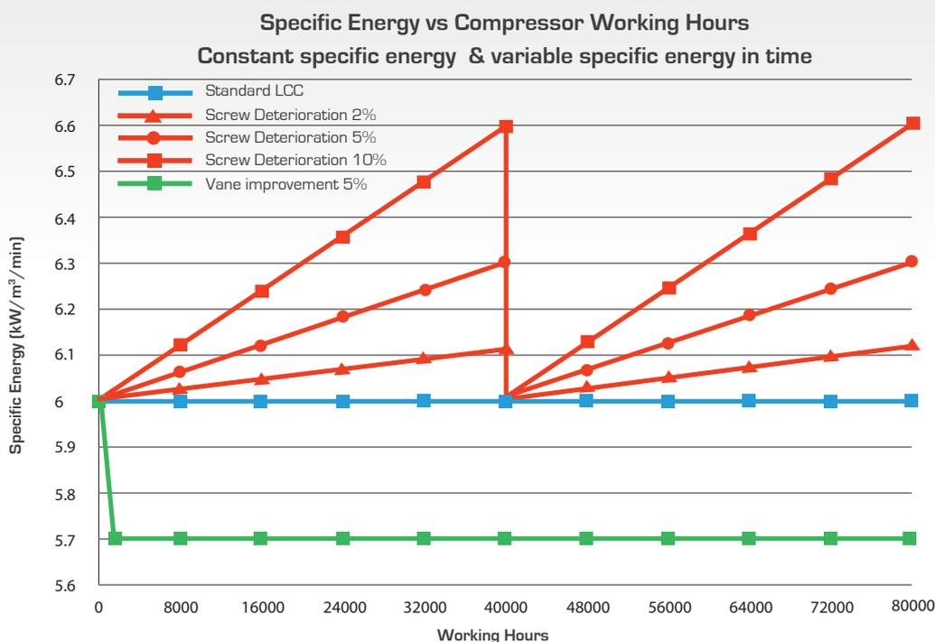
Fig. 12 - Changes in Specific energy over Compressor Working hours for various screw performance degradations over ten years with Compressor Overhaul at 40k hrs
