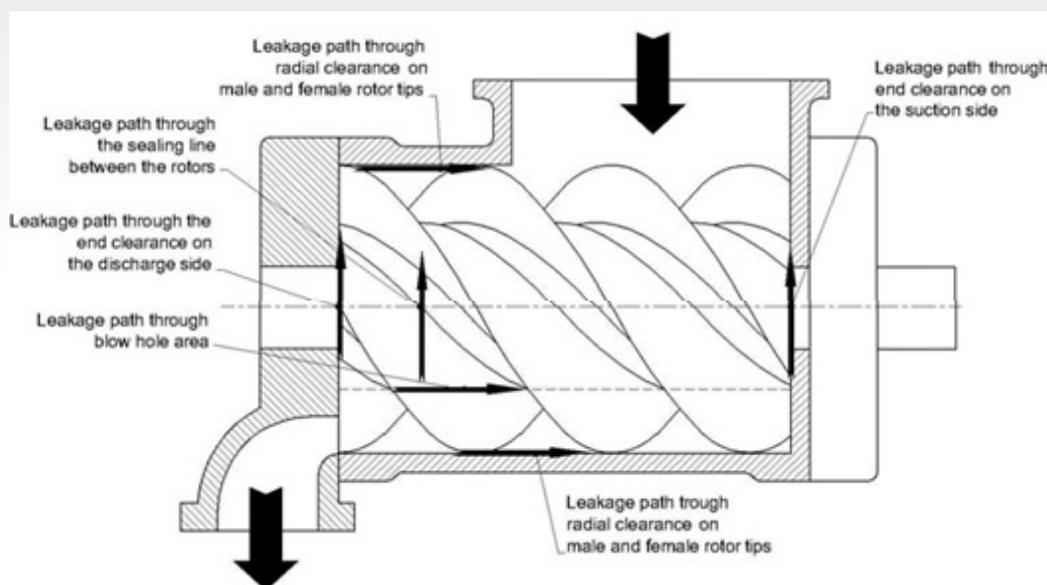
Fig. 5 - Leakage pathways in a screw compressor
