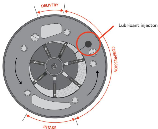
**Fig. 7** - The lubricant injected into the stator lubricates the moving parts and absorbs the heat of compression. All operational clearances (ends of rotor and blade tips) are completely sealed with the lubricant preventing high to low pressure leakage
