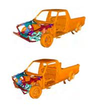
The refined final geometry is subsequently evaluated in an FE analysis.
