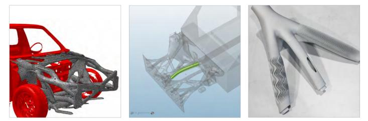
Bionic optimized design based on topology optimization results. Function integration enables to cut down the overall number of parts.
