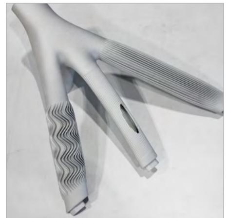
*Bionic optimized design based on topology optimization results. Function integration enables to cut down the overall number of parts.*
