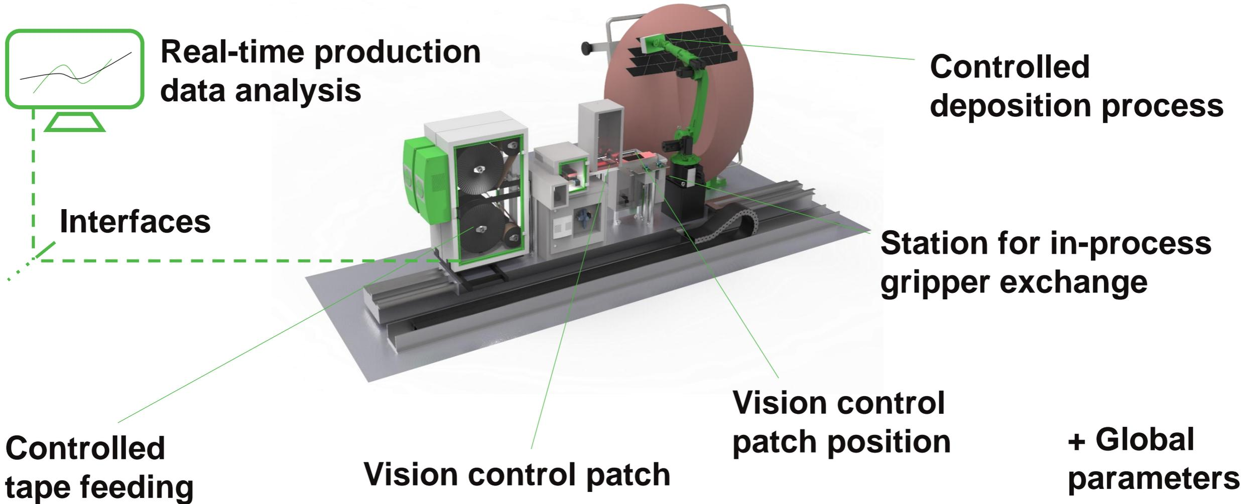
**Objective: Replace individual unit tests by continuous process monitoring**
