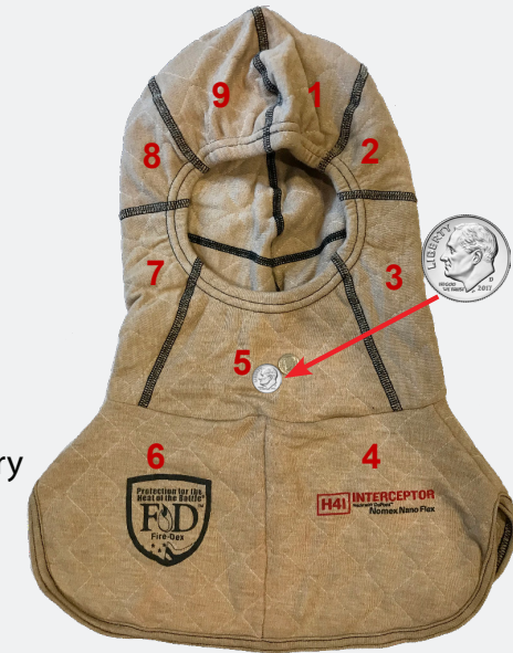
PANELS SEPARATED BY SEAMS (Numbers indicate visible panels: 11 Total)
