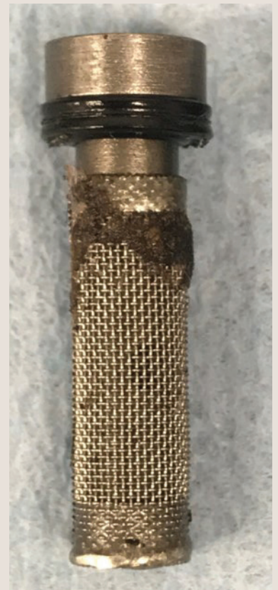
Inline filter as found
