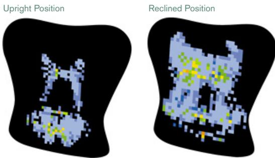
/ Figure 2 / In testing of both large, heavy users and small, light users, no pressure points (which would appear as red dots) are detected against Mirra 2's Butterfly Back, even when users are in reclined positions.
