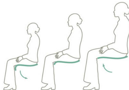
/ Figure 3 / If the front edge of a chair seat hits the user's thighs at the wrong spot, it can constrict blood flow and invite muscle pain. A 2.2 inch (5.6 cm) seat depth adjustment accommodates a variety of buttock-popliteal lengths with the ability to fit the seat depth to the body.
