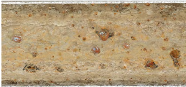
Zinc Oxide and Iron Oxide Deposits on Bottom of Main
