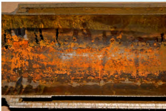
4 inch ECS In-Line Detector after 8 weeks exposure to compressed air (As Received)
