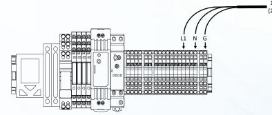
120v/1 Phase 60 Hz Connections (230v/1 Phase 50 Hz Connections)
