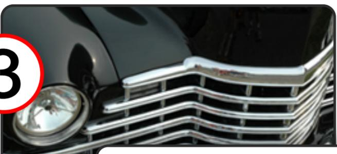
Martensitic steel contains approximately 13% chromium. Type 410 is a widely used, low-cost, general purpose steel used for applications where corrosion potential is moderate.
