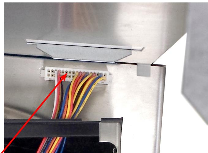
Connect wiring harness to the top of Cooler. Ensure all pins line up.
