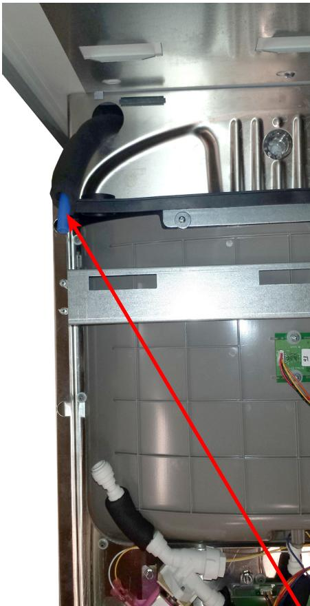
Fish 3/8 inch water line up through basin hole and hole in gasket.
