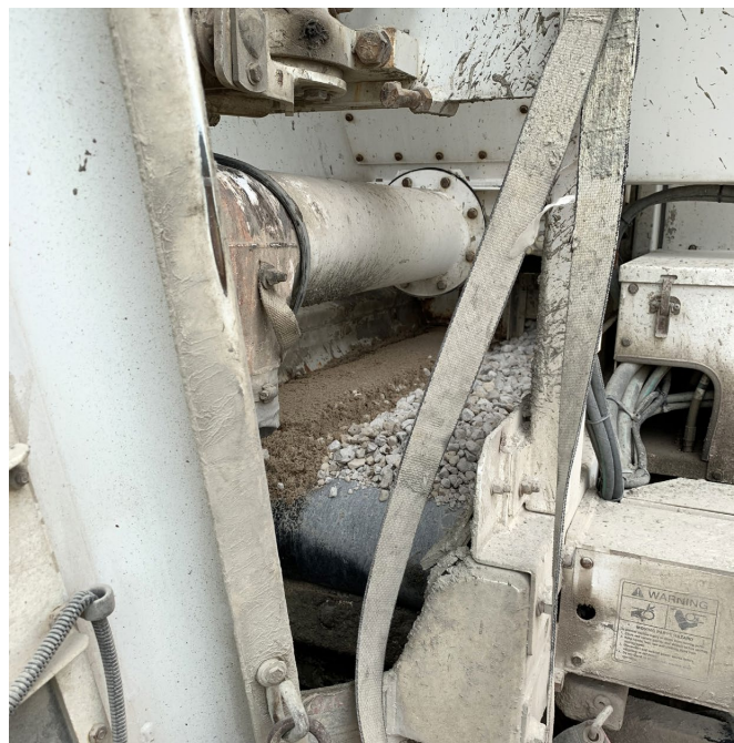
FIGURE 2: Constituent materials in the volumetric concrete truck's conveyor.
