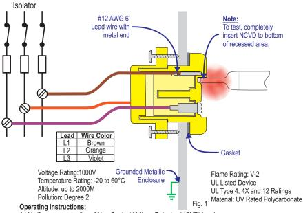
1.) Verify proper operation of Non-Contact Voltage Detector (NCVD) to a known source. With the Isolator closed and the electrical panel powered, verify the NCVD indicates voltage when completely inserted into the bottom of the recessed area of the R-T3 interface (figure 1). If the NCVD does not indicate voltage, then proceed with Lockout/Tag-out (LOTO) procedure as per NFPA 70E Annex G or other approved procedure.
