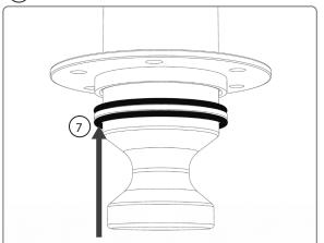
Place the bottom O-ring below the horn flange;
