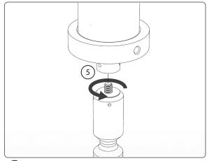
Thread the horn into the transducer by hand;
