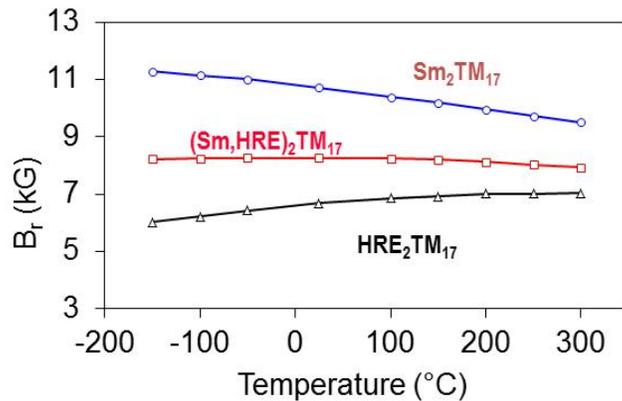
**Temperature dependence of residual induction  $B_r$  for  $Sm_2TM_{17}$ ,  $(Sm,HRE)_2TM_{17}$  and  $HRE_2TM_{17}$  magnets (TM=transition metals, HRE=heavy rare earth)**
