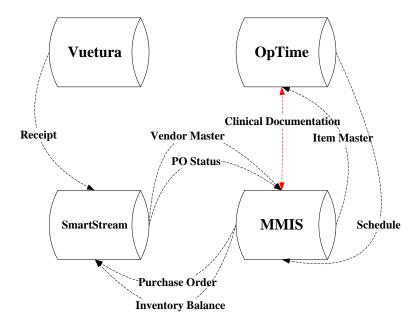
The diagram depicts the interface exchanges that will occur among the four systems. The diagram above depicts inbound and outbound interfaces from the various systems interacting with the IMIS. Outbound interfaces are represented by arrows leaving the system; incoming arrows are meant to represent an inbound interface to the system.
