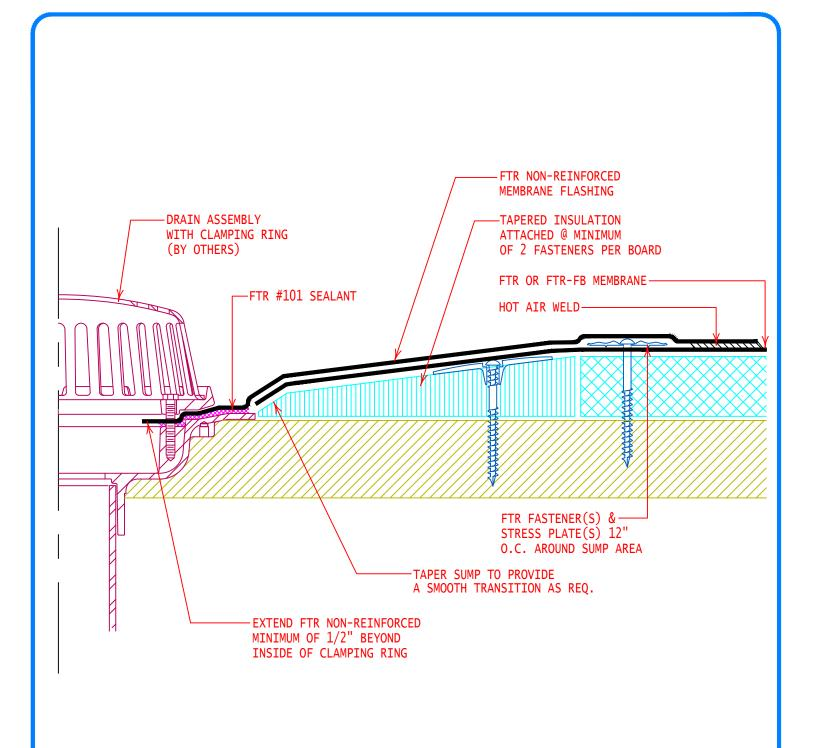
NOTE: USE TAPERED ROOF INSULATION (EDGE STRIPS) TO CREATE DRAIN SUMP. IF TOTAL INSULATION THICKNESS IS LESS THAN OR EQUAL TO 1 1/2 IN., TAPER 12 IN. FROM THE DRAIN CENTER. IF TOTAL INSULATION THICKNESS IS GREATER THAN 1 1/2 IN., TAPER 18 IN. FROM DRAIN CENTER.
