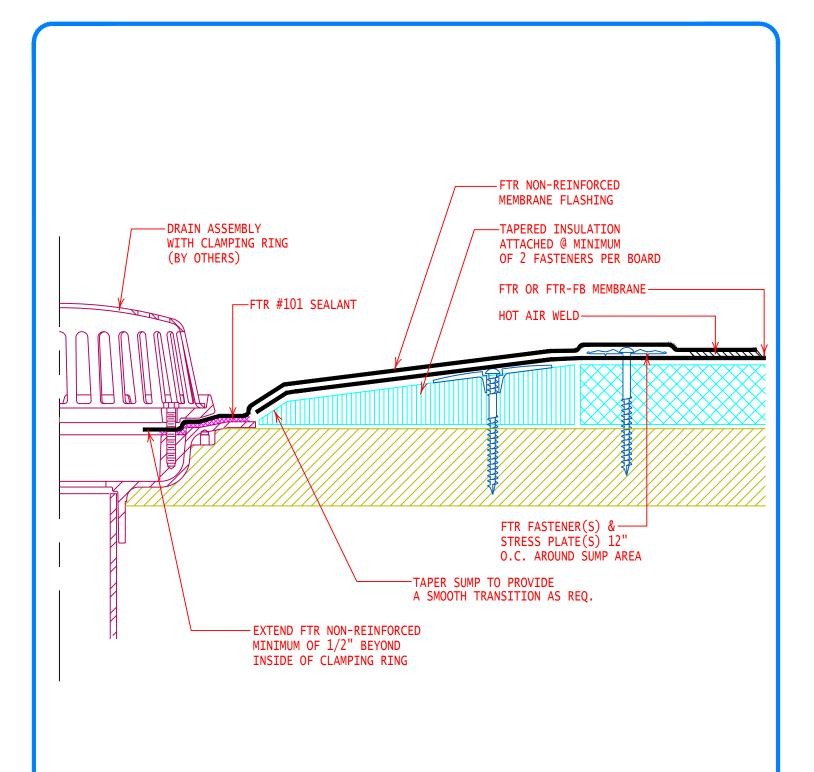
NOTE: USE TAPERED ROOF INSULATION (EDGE STRIPS) TO CREATE DRAIN SUMP. IF TOTAL INSULATION THICKNESS IS LESS THAN OR EQUAL TO 1 1/2 IN., TAPER 12 IN. FROM THE DRAIN CENTER. IF TOTAL INSULATION THICKNESS IS GREATER THAN 1 1/2 IN., TAPER 18 IN. FROM DRAIN CENTER.
