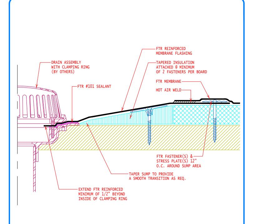
NOTE: USE TAPERED ROOF INSULATION (EDGE STRIPS) TO CREATE DRAIN SUMP. IF TOTAL INSULATION THICKNESS IS LESS THAN OR EQUAL TO 1 1/2 IN., TAPER 12 IN. FROM THE DRAIN CENTER. IF TOTAL INSULATION THICKNESS IS GREATER THAN 1 1/2 IN., TAPER 18 IN. FROM DRAIN CENTER.
