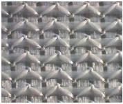
FiberTite's tightly knitted, high fiber content membranes exhibit characteristics similar to those of cloth or fabrics. It wants to lay on the roof more like a blanket as opposed to most "scrim" reinforced membranes.
