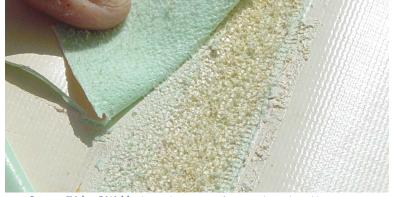
Poor or "Velcro" Weld indicates the presence of moisture during the welding process.
