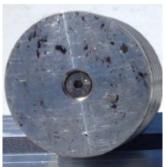
A dirty magnet should be cleaned before using.
