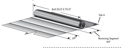
When pulling subsequent tabs, keep the core of the roll behind the previously fastened tab. Continue pulling down and attaching tabs in sequence.
