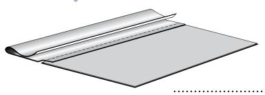
Now the membrane can folded in half to permit application of the adhesive to the substrate.
