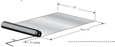
Roll the tail of the roll back to the core. Apply FTR 290; 390 or 490 adhesive to the substrate. Keep adhesive away from overlap areas. Allow the adhesive to set up to a point where it is still wet but sticky and mildly stringy to the touch. Evenly maneuver the membrane into the wet adhesive.
