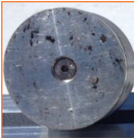
A dirty magnet should be cleaned before using.
