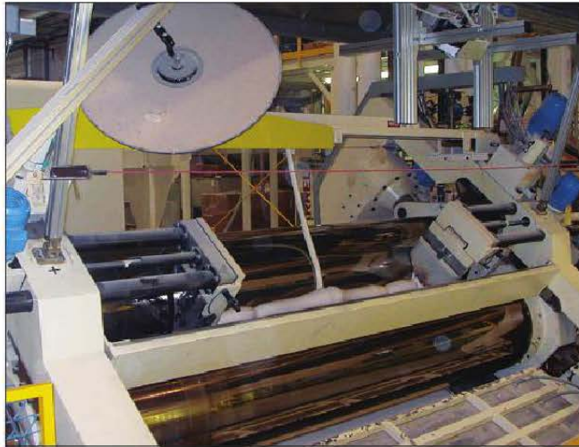
State-of-the-art hot-melt calendar for manufacturing KEE membranes.
