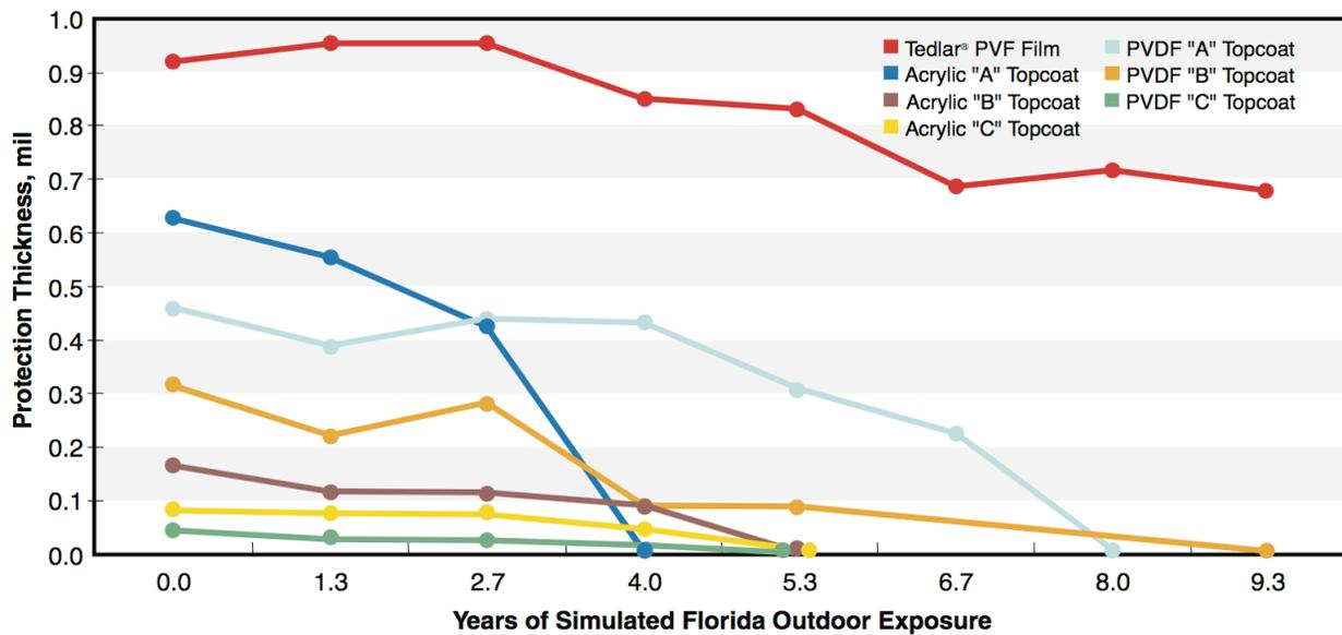
Note: This simulation shows that Tedlar® protective film not only starts out thicker than any of the other protective coatings, but retains superior thickness long after the others eroded completely.
