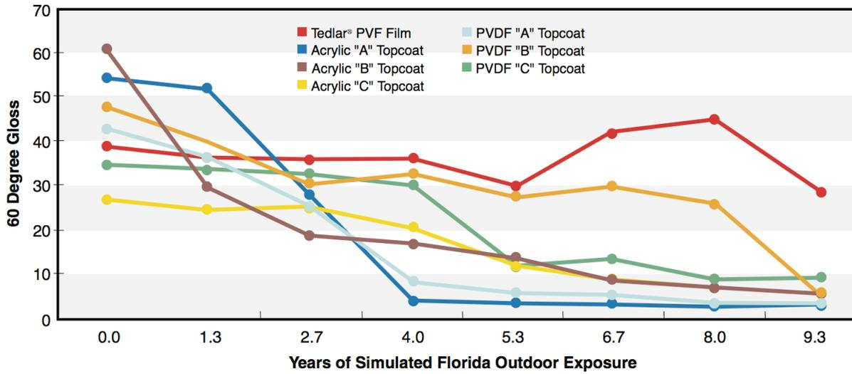
The Tedlar® PVF film shows excellent gloss retention after the equivalent of nearly 10 years of exposure, while the coating materials have failed to maintain their integrity. In fact, because the protective layers of the coating materials have been essentially depleted, both color and gloss measurements on these systems are probably the properties of the PVC substrate alone.
