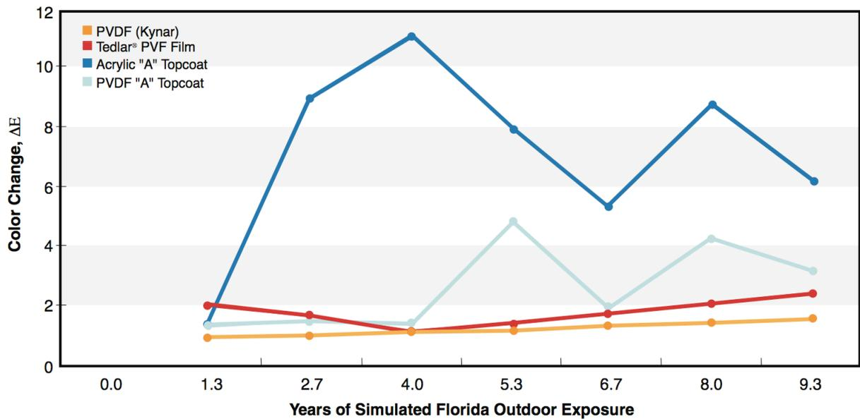
Color change can be attributed to degradation by UV light and dirt pickup. Note that the Tedlar® PVF film shows no color change after the equivalent of nearly 10 years of exposure.
