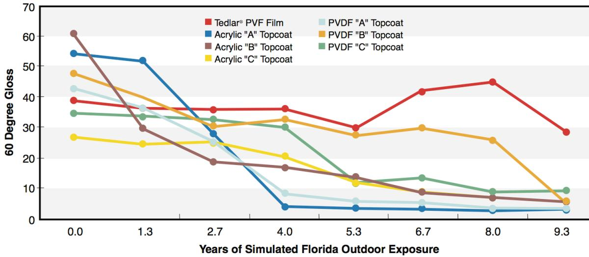
The Tedlar® PVF film shows excellent gloss retention after the equivalent of nearly 10 years of exposure, while the coating materials have failed to maintain their integrity. In fact, because the protective layers of the coating materials have been essentially depleted, both color and gloss measurements on these systems are probably the properties of the PVC substrate alone.
