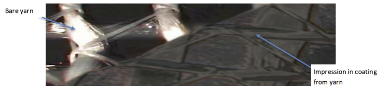
Figure 4. Laminate geomembrane with poor mechanical adhesion
