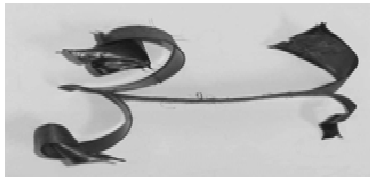
Figure 5. Inter-ply separation of unreinforced film
